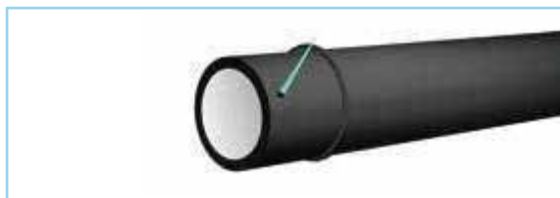
2. Greasing of the outside surface of the straight pipe end
