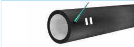
3. Greasing of the outside surface of the straight pipe end
